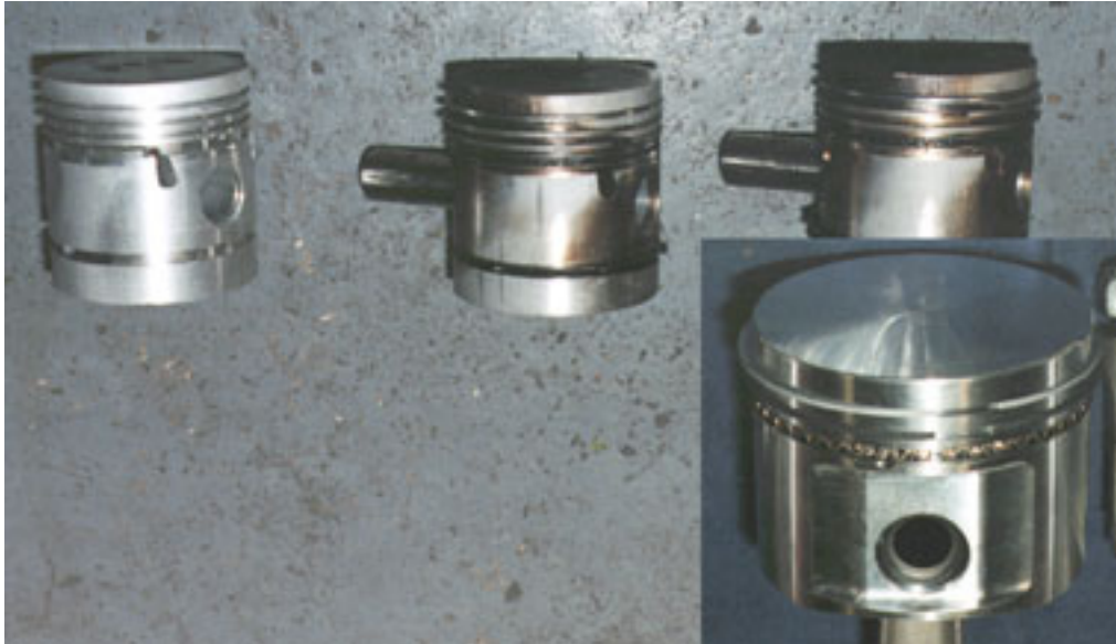
Piston in the lower right is the modern JE Piston. The others are original.
